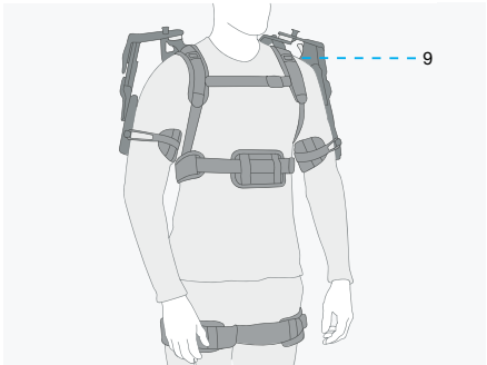
Back support module (C): 9. Activation mechanism
